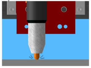
Typically you would want 3/16" retract distance as well as a static cutting distance between the tip and the material, although this can very between 1/8" to 1/4".
