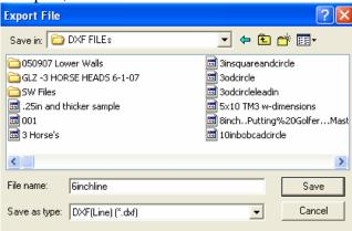
Then import this 6inchline.dxf file into the Torchmate 2 software. Once imported, zero out the program coordinates in order to cut this on your material.
