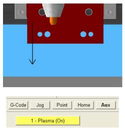
Once the torch has sensed the material and backed up to its pierce height, you can proceed to measure how far the torch actually retracted.
