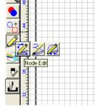
With one red cross node placed, on the top of the screen there are two white boxes. In the left box type in 6 and hit enter. This will draw a line with two nodes, 6" long.
